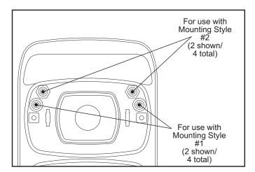
**Mounting Style #2** is best suited for applications where there is access to the backside of the mounting surface. The style requires 4, 1/4-20 Hex Head bolts, split-lock washers and nuts (customer provided). Bolts should be of a length appropriate for your specific installation.
